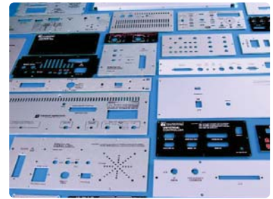
Custom punched holes in enclosure panels
